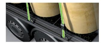
The anti-slip mats must be at least 150 mm wide and 3 mm thick. The length of the mat depends on the diameter of the coils. The anti-slip mats are positioned under the paper coils so that approx. 1 cm of mat can still be seen from the outside.
