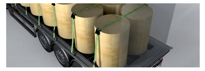
**Example** for calculating how to secure a load of upright paper coils without taking account of the load rating of the front end wall
