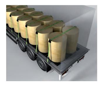
Please also note that even when taking account of the load rating of the front end wall with a total positive fit with no gaps, the paper coils still have to be strapped down when using **REGUPOL Anti-Slip Mats** even if theoretically no additional securing is necessary. After all, consideration also has to be given to dynamic vertical movements and the risk of the paper coils tipping over.
