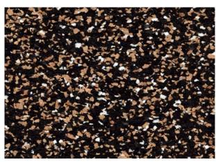
Regupol® 4515 4.5mm is manufactured from recycled PUR foam and cork
