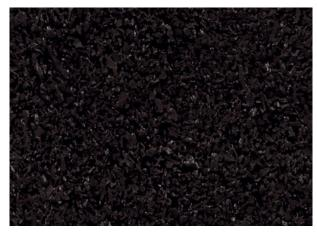
Regupol® 6010 is manufactured using recycled SBR rubber
