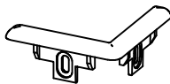
SM-20N END CAP - (24I068xxx, SHOWN) SM-20N CHAMELEON CAP - (24I646xxx) SM-10N END CAP - (24I126xxx) SM-10N CHAMELEON CAP - (24I993xxx) SSM-20N END CAP - (24I070xxx) SSM-20N CHAMELEON CAP - (24I622xxx)
