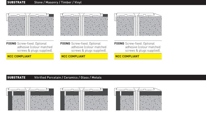
FIXING Screw-fixed. Optional adhesive (colour matched screws & plugs supplied). NOTE Ensure grout line is discrete as illustrated
